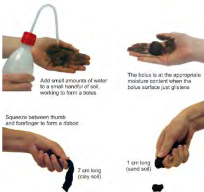
Figure 2. Formation of a ball and ribbon to determine soil texture. (Source: Anderson et al., 2007)
