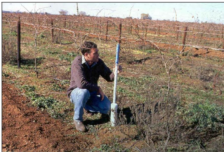
**Figure 11.** Testwell in vineyard with capacitance logger
