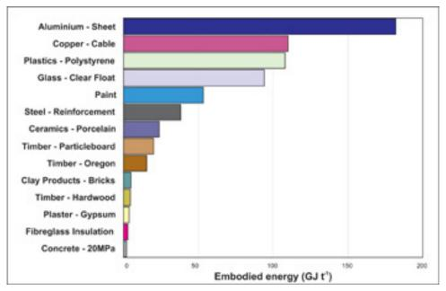
Figure 4. Embodied energy (GJ/t) of various building materials [2]
